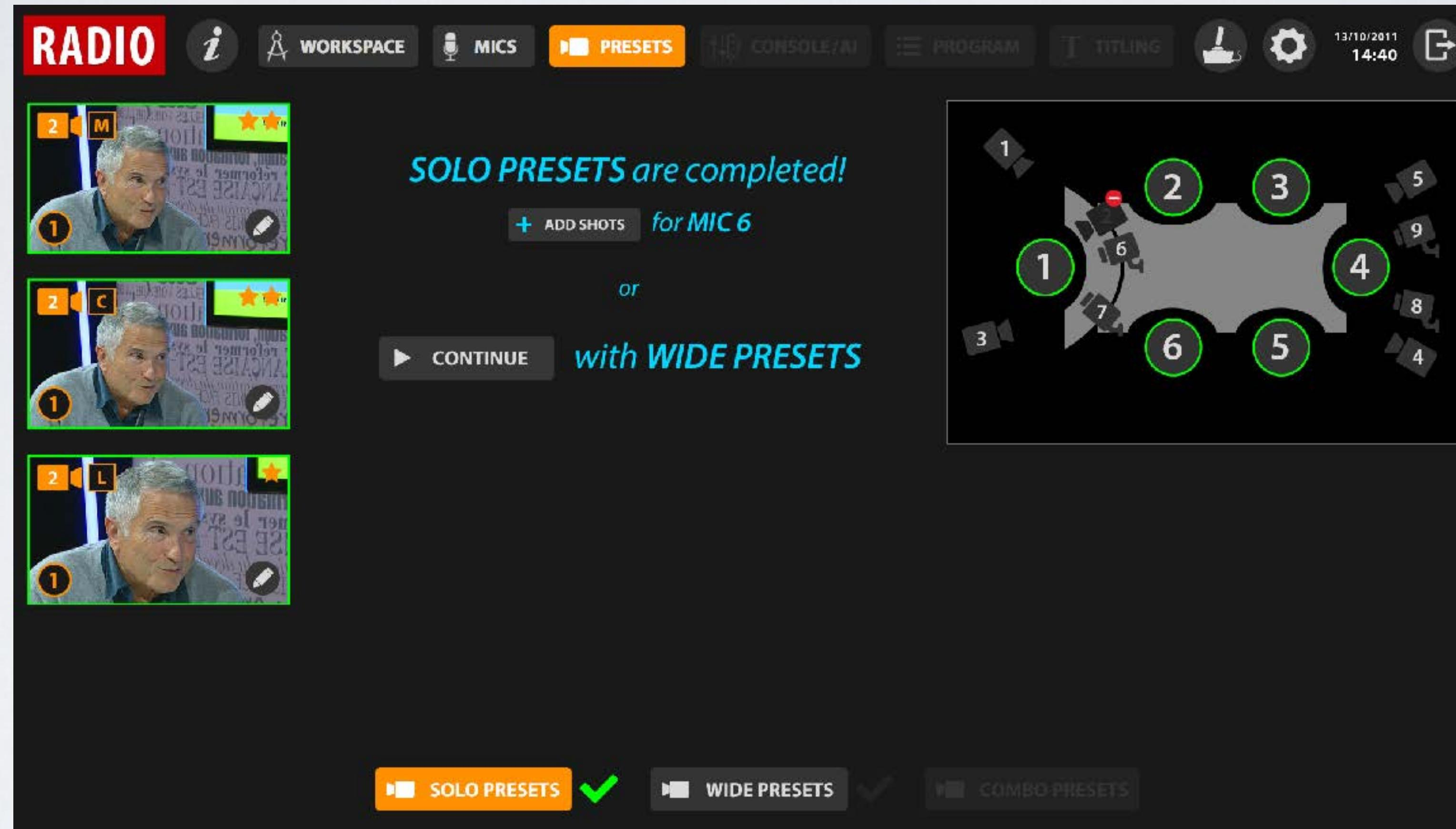
Each microphone is covered by **different angles of shots** with the PTZ cameras installed in the radio studio
